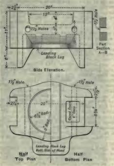
Fig. 4.—Cast-Iron Follower for Driving Steel Sheet Piles.
